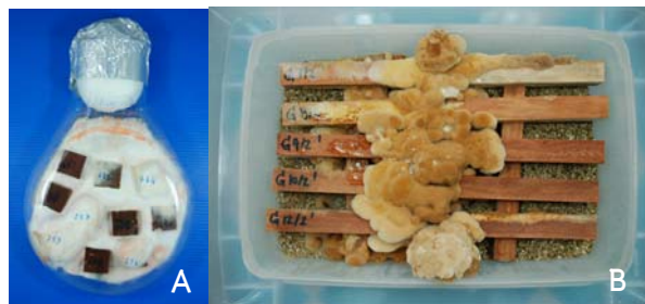
Figure 5. Experimental method (A) Agar block test and (B) Wood stick sandwich method.
